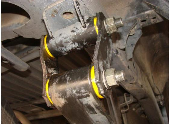
I lowered the front leaf spring/bushing, was secured by the dreaded 23mm nut. My only 23mm socket is a deep impact one, and there wasn't enough clearance to use that, the fuel tank was in the way. So I used a (shoot me) 12 inch adjustable wrench. Anyway, the front bushings looked pretty good, and I wasn't able to remove those as easily as the rears, so I decided to leave those as OK. I bent the two U-bolts a little tighter in the bench vise, so I could feed them into the lower bracket.
