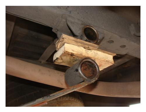
I was able to readily remove ALL the rear bushings by hand, that saved a lot of time. I cleaned up the "cylinders" where the bushings sit using steel wool. I greased two of the bushings and the shackle surfaces and the internal surface of the "cylinders" and put the bushings onto the shackle.
