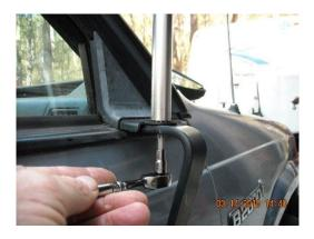
You can also use thread locker on the T30 bolt to make sure it doesn't come loose in the future, the key is to keep the head to pole connection lubricated every so often. I used white lithium grease when sliding the head back on the pole. Uhhh, that sounded dirty!:rollinglaugh:
