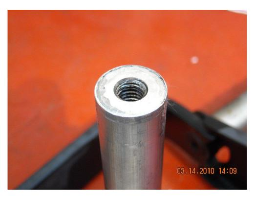
I took a file and laid it on the workbench and then drug the end of the pole across the file while trying to keep it perpendicular to the file so I could flatten the mounting base of the aluminum pole out and have it grip better when I tightened it down for good, hopefully. I also used some red high strength thread locker on the T30 bolt on the drivers side mirror. The passenger side was still tight and hadn't slipped yet.
