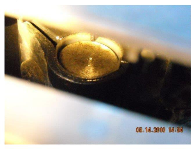
Pull up on the mirror head while slowly twisting it back and forth and you should be able to pull the whole mirror head off the aluminum pole.
