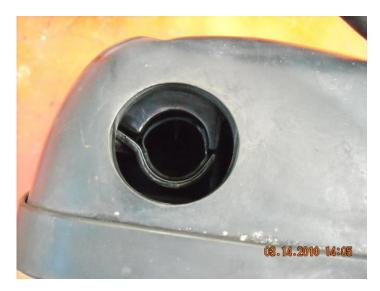
My drivers side was real loose at the T30 bolt connection.....the bolt wasn't loose, it was loose because it had started rotating at the T30 bolt and the star washer had started to eat up the base of the aluminum pole.
