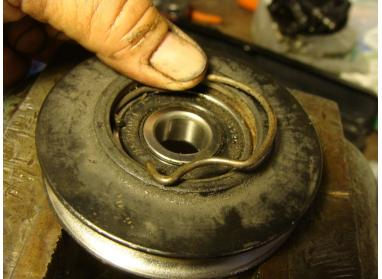
Use a socket (I used 9/16 impact socket) and hammer to tap the old bearing out.
