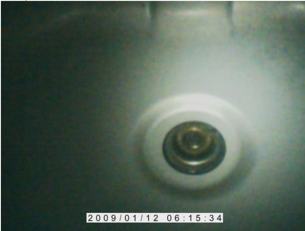
Photo of inside of fuel tank, using special inspection camera, a gift from daughter. Photo shows no rust or debris, GOOD !!!
